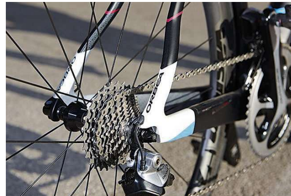
▼ The internal cable routing through the chainstay for the Dura-Ace Di2 drivetrain is as neat as it gets
